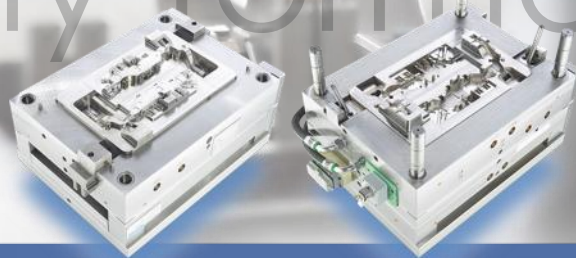
2-cavity injection mold with hot runner, 2 sliders, 2 core pullers and overmolded metal inserts
