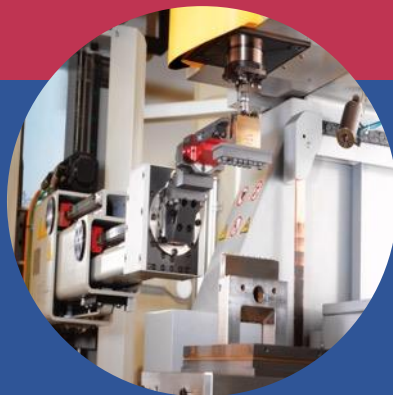
Fully automated change of sinking electrodes and workpieces by robot system
